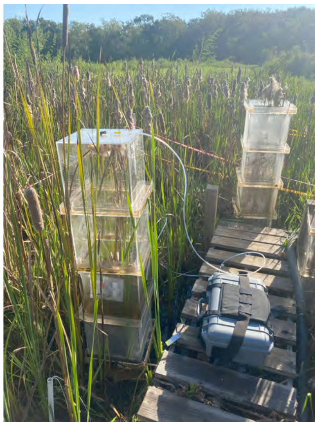
Chamber for greenhouse gas flux measurements in wetlands.
